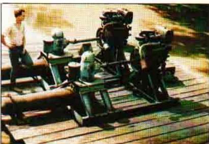
Model 9/9 floating pumps operating as emergency stand-by pumps for the Malaysian Agricultural Development Authority.
