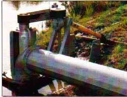
A portable, tractor driven model 11/11 used in this application as a drainage pump to extract 225 litres/second with 4 metres Total Dynamic Head.
