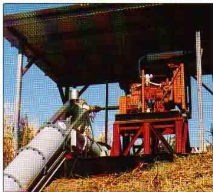
The model 21/24 Angle Application pump used for cotton irrigation, operating at Moree, NSW, Australia. This system pumps 1000 litres/sec at 6 metres Total Dynamic Head.
