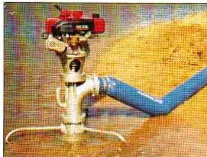
A portable petrol driven pump from the Portax series which extracts 30 litres/second, Colombo, Sri Lanka.
