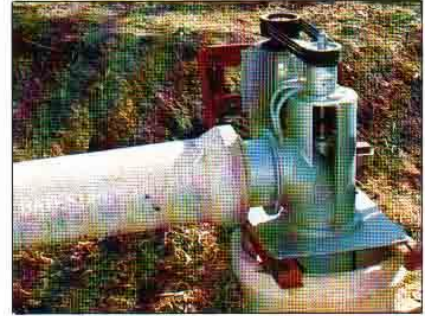
This model 11/14 irrigation system pumps 225 litres/second with 5 metres Total Dynamic Head and is used to supply rice fields.
