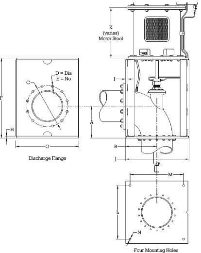
Head size = nominal bore;  $\vec{E}$  = No of holes in discharge flange.
