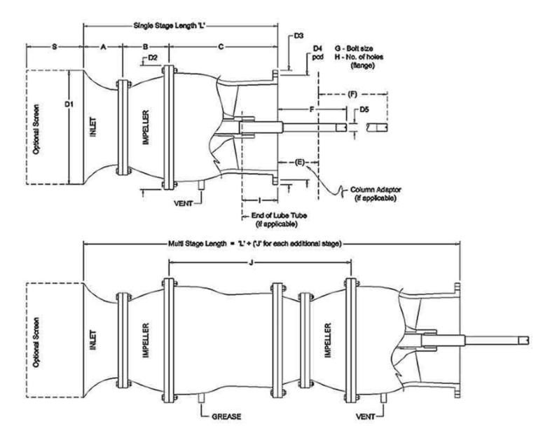
Note: Pumps 14MC & 14MD have the same external dimensions, differing only in impeller design.
